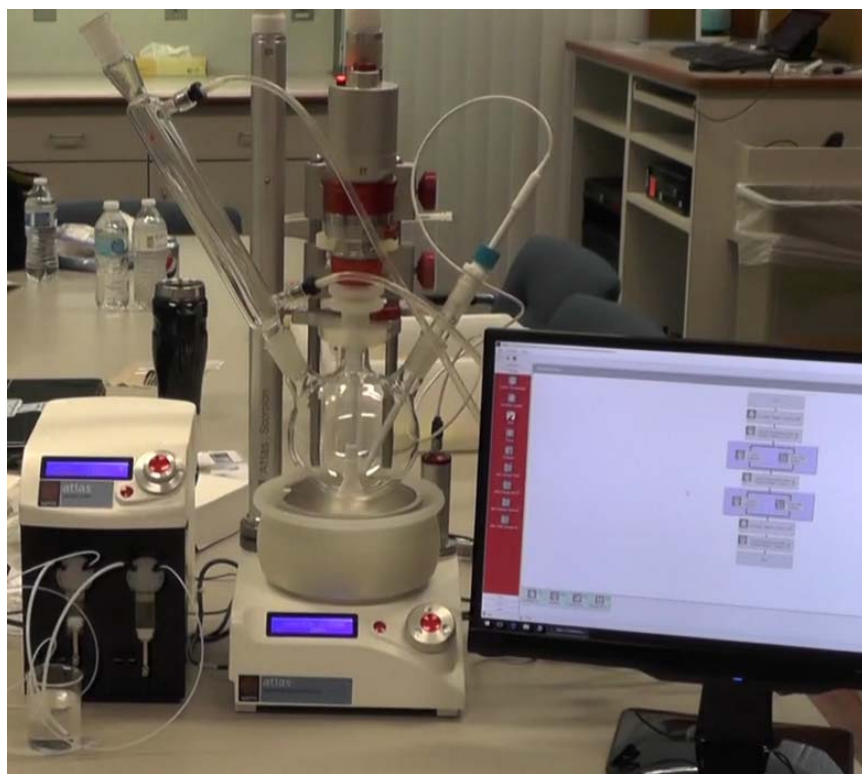
Figure 1. Photograph of Atlas batch chemistry system during training and programming of magnetite core protocol into Atlas software.
